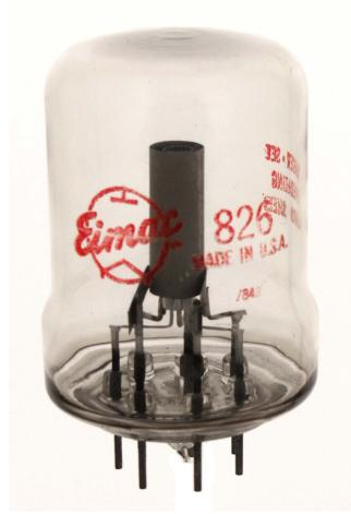
Eimac made a few of these tubes. Recently a pair of experimental tubes was found that seemed to be an attempt to use the basic 826 with a heavy plate structure and equip it with a plate cap. The plate was massive for the size and
