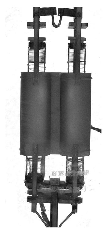
The unusual feature of this tube is that the elements are made in two parallel sections. This construction wasn't needed to produce the required power, but if you look at the construction, it seems to be for ruggedness. I can imagine that electronics equipment in WWII was subjected to very rough treatment in transit. I have problems with the USPS and UPS shipping tubes and conditions in the Pa-
