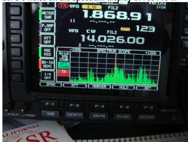
20/ S-9 noise on the spectrum display of 756 Pro III
