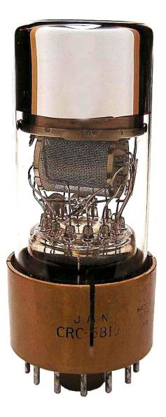
The multiplication process can result in a signal 1,000,000 times the input.
