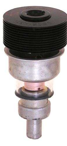
Later versions were rated at 100 watts and 2.5 GHz+. They came with both glass and ceramic insulators. The military liked them for pulse operation so they were made with longer ceramic insulators to handle the high voltage. The most common use for them commercially was in 450 MHz 2-way radio. The first FCC type approved 2-way radios were Motorola
