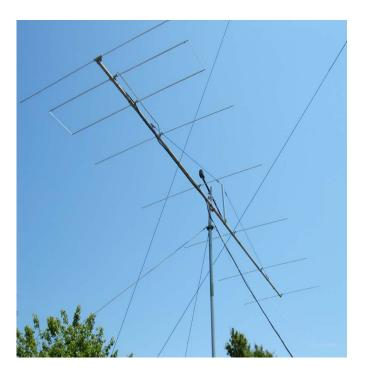
When the antenna was assembled and tested it looked very good electrically. The antenna rotor was too small and couldn't handle the long boom. A Ham4 rotor was borrowed from W6SR, but it proved too heavy and the mast almost fell over. The antenna was designed for high elevation adjustment using an actuator arm like they use on small TV dishes.
