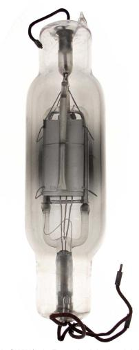
After the end of WW1, de Forest had the legal right to produce transmitting tubes and made a series of high power oscillions. These were usually 250 and 500 watt dissipation versions. The tubes were designed to operate in ver-
