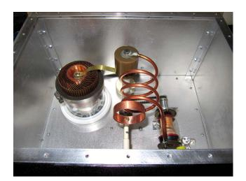
**The new GS-35B** amplifier for 6 meter EME is complete and testing has started.
