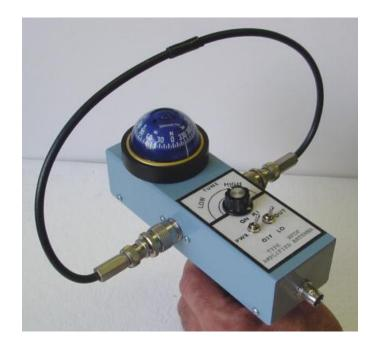
The Vector Gun includes a switchable high-gain amplifier and a switchable attenuator, along with five loops covering 1.8 to 55 MHz. Alan uses this device, paired with either a general coverage portable receiver with a signal strength meter or a SDRPlay, to track down interference.
