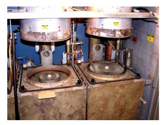
The 8891 and its driver tube were mounted in a pair of silver plated, tunable cavities. The tube sockets were made with many finger stock contacts that needed to be cleaned or re-plated periodically. The cavities needed to be disassembled to get to the sockets. When the sockets were re-assembled, the alignment tool shown was used to keep the filament and grid rings in perfect symmetry.
