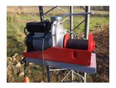
After I bolted the hoist to the shelf I made sure the cable was wound on the reel correctly, then tested it to make sure it lifted and lowered correctly. It takes approximately 30 seconds to raise or lower.
