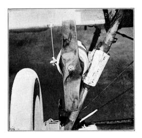
The generator assembly was mounted on one of the landing struts. The photos were taken by the Signal Corps in about 1918.
