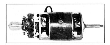
If the plane was flown too slowly, the generator wouldn't make enough voltage and if flown too fast the voltage would be too high and possibly smoke the regulator. They found that 4000 to 14000 r.p.m. would work correctly. That r.p.m. translated into air speed was 50 to 200 miles per hour.
